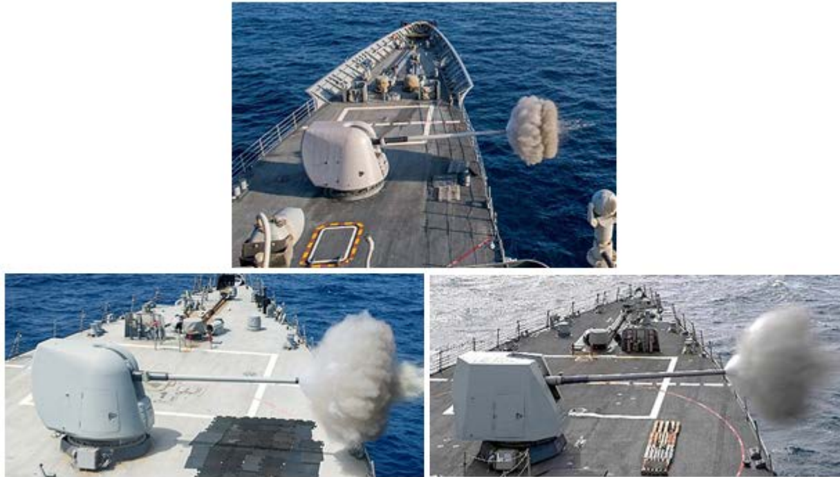
Figure 3.0-1: Gun Blast and Projectile from a MK 45 MOD 2 5-inch/54 Caliber Navy Gun on a Cruiser (top), a MK 45 MOD 2 5-in/54 Caliber Navy Gun on a Destroyer (bottom left), and a MK 45 MOD 4 5-inch/62 Caliber Navy Gun on a Destroyer (bottom right)
